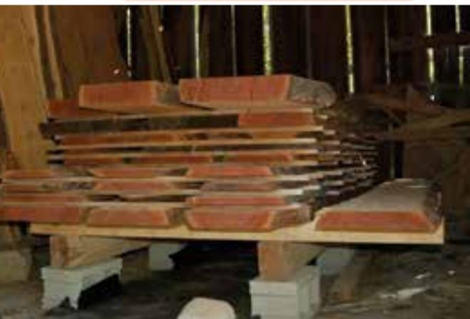
For those like me who want to air dry their wood, it is essential to start by building a good foundation off the ground, properly separate the uniform layers of boards or flitches with stickers, and make sure the stack is covered, or better yet, under some sort of roof. It is also best to dry in a mostly shady location and not subject to strong winds.
