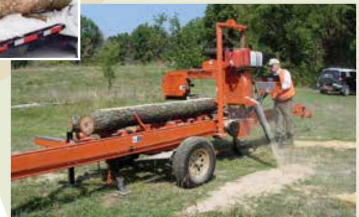
My saw has easy set-up, a heavy steel frame and trailer, and a large engine. The manual model has a winch that can be used to roll logs onto the mill, but I prefer to carefully load logs by rolling or sliding them off the tractor forks. I use a cant hook to position and turn the logs.
